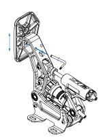
The Formula Version can be adjusted at two different heights thanks to the two M5x10 countersunk screws on the front of the pad using the TX25 key. Holding still the nuts on the other side with the supplied wrench, simply remove the screws and you're good to go.
